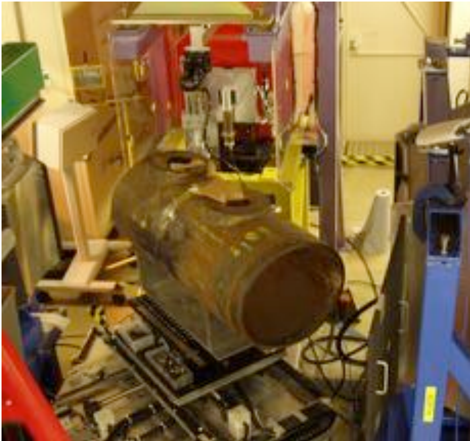
Welded pipe on Engin-X
